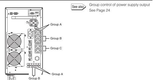
Procedure for connection to power supply output receptacle (IEC60320 C13)
